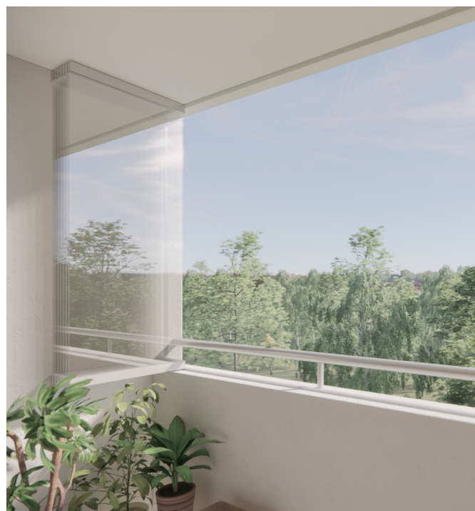
Balcony with folding glass: The drawing shows how the balcony can be used as an open balcony when the folding glass is pushed to one side. Note: Subject to changes
